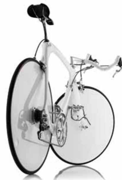
Bianchi C-4 Project, c.1988 Debuted in the 1987 Giro, the Project is the product of two polar opposites: Bianchi, a traditionalist's bicycle manufacturer dating back to 1885, and C-4, a cutting edge composites outfit founded some hundred years later. The Project's most striking feature is its lack of seat tube and
